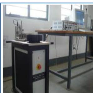
Figure 3. Over All View of the Pin-On-Disc Machine
