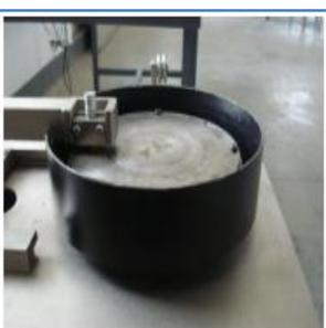
Figure 4. Pin and Disc Arrangement
